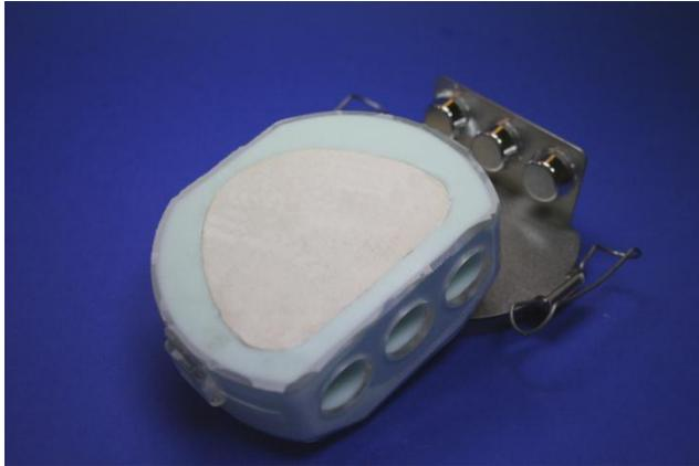
9) Mix the resin according to the manufacturers' instructions. The flask has to be filled by a thin jet only through the middle canal till it comes out of the other canals. Afterwards put the flask into the pressure pot 2.5 bar for about 25 min at 45 °C water temperature.
